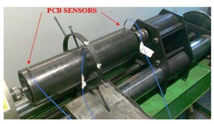
Fig. 3. Test stand with mounted roller and accelerometers
